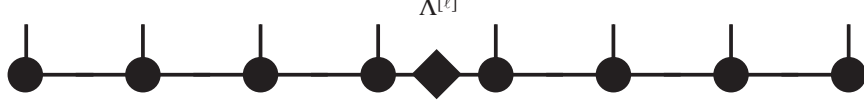
Figure 59: MPS structure generated by infinite-system DMRG at step \ell : a string of left-normalized A , a string of right-normalized B , joined by a diagonal singular value matrix \Lambda^{[\ell]} . Note that structurally the central unit does not repeat.
